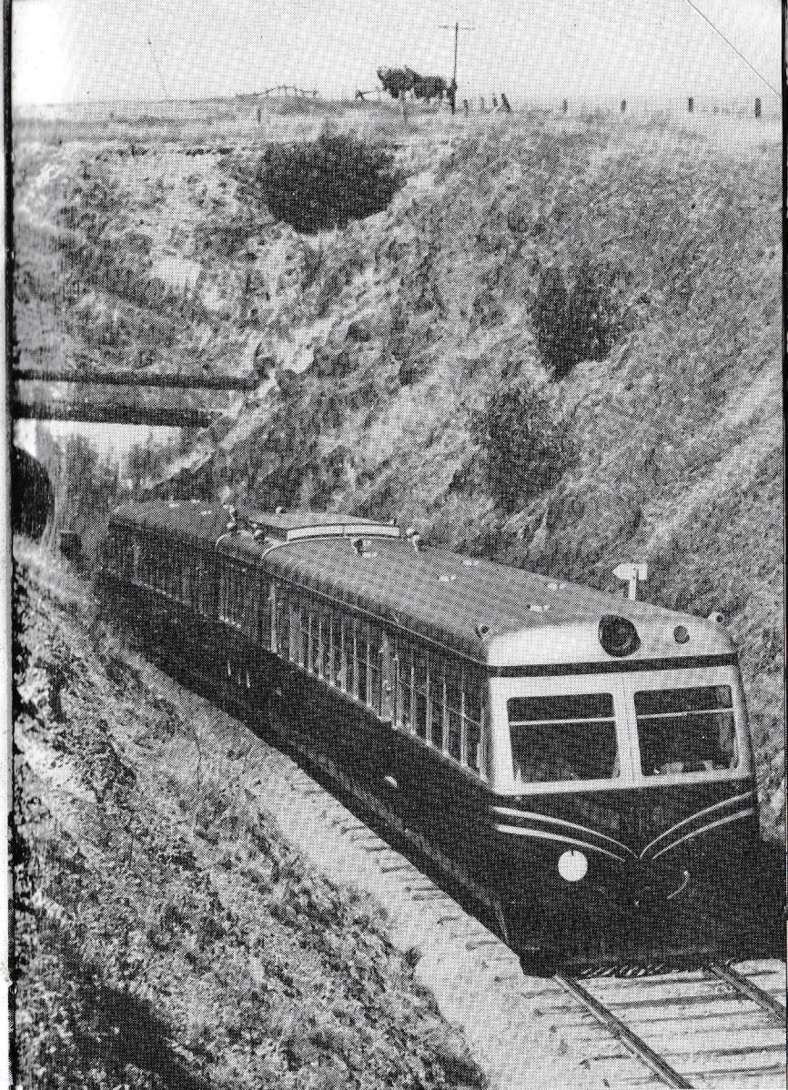
280 h.p. diesel rail-car on the Mansfield line
